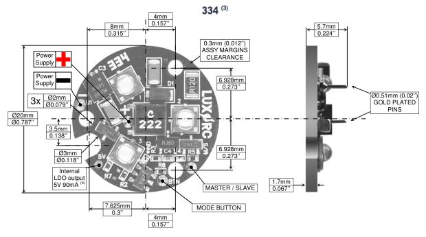
Note 3: The 334 should be installed on a flat clear heat sink. The engine can be either glued using a thermally conductive adhesive or fastened by a ring or nut. We recommend applying DOW CORNING 1-4173 thermally conductive adhesive or similar to minimize thermal resistance and attain maximum performance.
